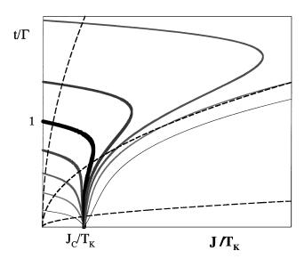
FIG. 2. Schematic contour map of the conductance in the  $N \simeq 2$  regime. Thicker lines denote higher conductance, the thickest one corresponding to  $g = e^2/h$ . The broken lines are three physical contours (for different values of  $\alpha \equiv \Gamma^2/UT_K^0$ ) along which  $J \sim t^2/U$ .
