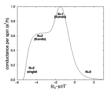
FIG. 3. Plot of the conductance versus the level energy, as obtained from SBMFT (for t = 2 and  $U/\Gamma = 10^4$ ). The conductance rises from a very small value (the singlet regime,  $J \gg T_K$ ), to a *t*-dependent value (N = 2 Kondo regime,  $J \ll T_K$ ), and then to  $g = e^2/h$  (N = 1 Kondo regime) before dropping to zero for an empty dot.
