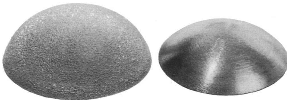
Fig. 9.32. Rough as-grown outer surface of CVD diamond dome and appearance after machining to a roughness of 1\ \mu\text{m} with a Nd:YAG laser. The laser-machined dome appears black because the surface is converted to a thin layer of graphite which can be easily removed by subsequent polishing. [Raytheon photos courtesy C. B. Willingham.]
