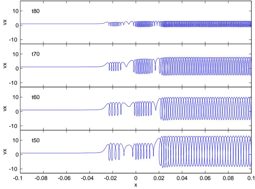
**Fig. 2.** Trajectory of a single electron with the initial velocity  $\mathbf{v}_i = (V_u, 0, V_u \tan \theta)$  in the de Hoffman-Teller frame for several values of the angle between the shock normal and upstream magnetic field. The Mach number  $M = 6$ , magnetic compression  $B_d/B_u = 3.5$ , de Hoffman-Teller cross-shock potential  $e\varphi_0 = 0.15(m_i V_u^2/2)$ , and shock width  $\approx 0.4(c/\omega_{pi})$  are the same for all cases.
