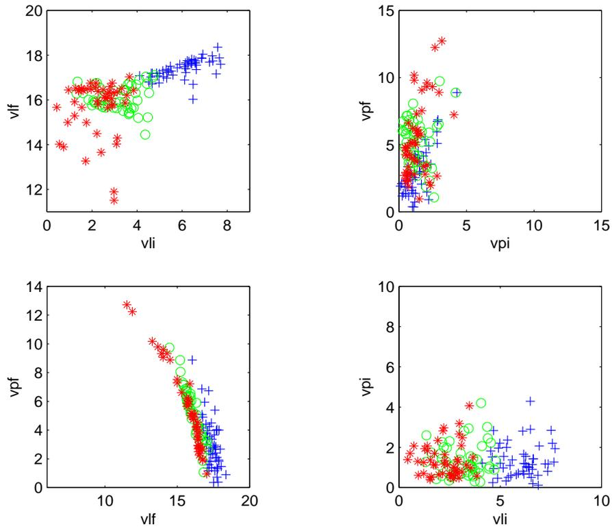
**Fig. 4.** Liouville mapping for 50 electrons (initially Maxwellian distributed with  $\beta_e = 0.05$ ) for  $\theta = 80^\circ$  (crosses),  $\theta = 70^\circ$  (circles), and  $\theta = 60^\circ$  (stars).
