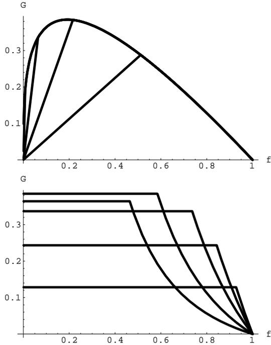
**Figure 8.** Gain as a function of frequency,  $\xi = \omega/\omega_{r0}$  (left panel), and opening angle,  $\eta = 3\gamma_b\phi_0/8$  (right panel).
