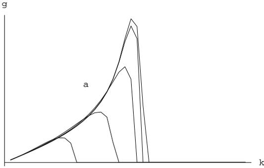
**Figure 1.** Growth rate vs frequency for the cold-cold case and different angles of propagation. The instability range squeezes as the propagation angle increases: higher growth rates and larger regions of instability correspond to smaller propagation angles.
