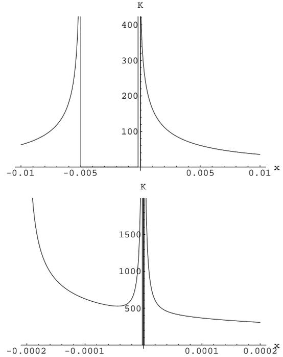
**Figure 3.** (Left)  $K$  as a function of  $x$  for the double waterbag case with  $\alpha = 0.1$ ,  $\theta = 0.1^\circ$ ,  $\gamma_1 = 10$ ,  $\gamma_2 = 50$ ,  $\gamma_3 = 500$ , and  $\gamma_4 = 1000$ ; (Right) The instability region magnified.
