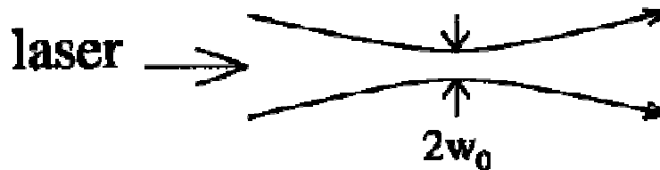
FIGURE 11.1. A single focused laser beam produces the simplest type of optical trap.
