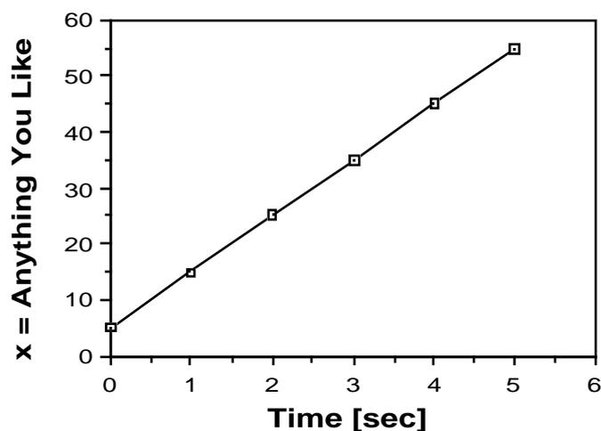
**Figure 1:** Graph of "anything" vs. time. If "anything" represents *position*, the slope of the graph gives the object's velocity. If "anything" represents *velocity*, the slope of the graph gives the object's acceleration.
