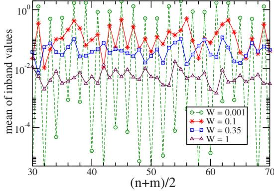
FIG. 6. (Color online) The mean of the in-band values of the  $|v_{nm}|^2$  matrix elements as a function of  $(n+m)/2$  for different values of disorder. The pronounced modulation in the ballistic regime is an indication for texture.
