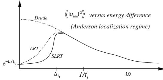
FIG. 8. Schematic plot that illustrates the dependence of the average and the typical values of the matrix elements on the energy separation  $\omega$ . These are labeled as “LRT” and “SLRT,” respectively, and compared with the semiclassical (Drude) expectation. The plot refers to the Anderson regime. For a corresponding numerical illustration in the ballistic regime see Fig. 7.
