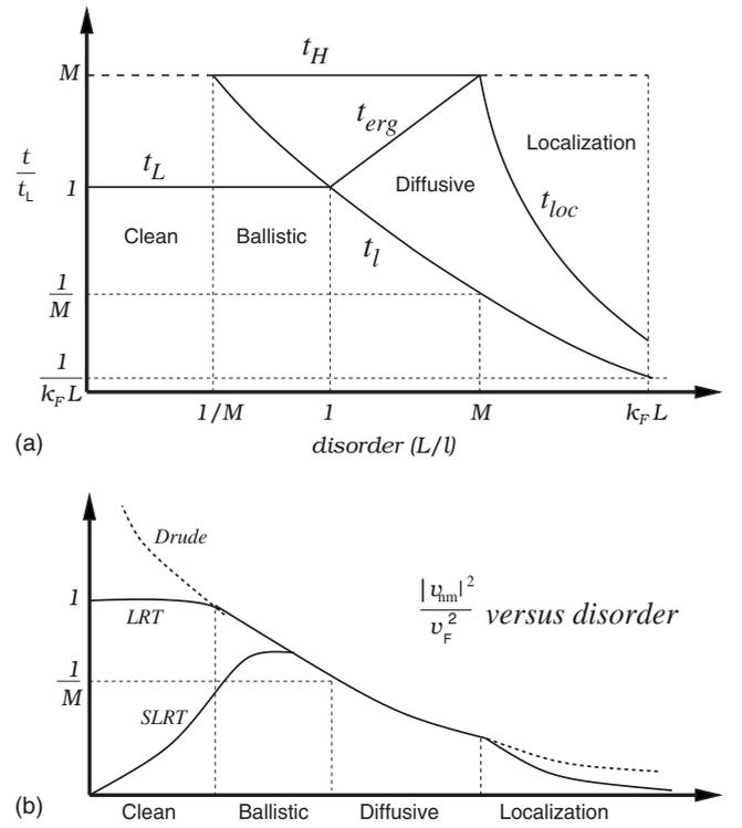
FIG. 4. Upper panel: time scales versus the disorder strength (see Sec. II A). Lower panel: schematic illustration that sketches the dependence of the dc conductance on the strength of the disorder. It should be regarded as a caricature of Fig. 2.
