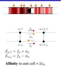
$$\begin{split} \boldsymbol{W} &= \boldsymbol{\sigma}_{\boldsymbol{x}} + \boldsymbol{W}_{\text{hop}} - \sum_{n,s} |n,s\rangle \, \gamma_{n,s} \langle n,s| \\ \boldsymbol{W}_{\text{hop}} &= \sum_{n,s} |n+1,s\rangle \langle n,s| \, e^{\frac{\mathcal{E}_{n,s}}{2}} + |n,s\rangle \langle n+1,s| \, e^{-\frac{\mathcal{E}_{n,s}}{2}} \\ \end{split}$$
