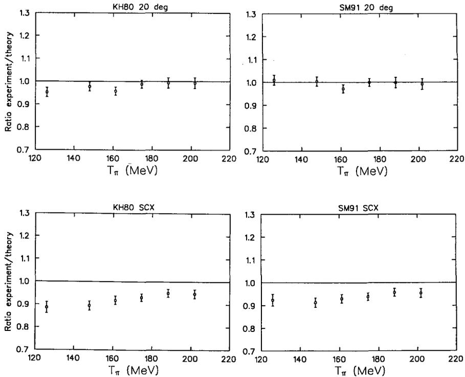
Fig. 2. Comparisons between the present experimental results and predictions made with the KH80 [13] and SM91 [12] sets of phase shifts. The lower half refers to the SCX cross section. The top half refers to the measured “partial–total” cross sections in comparison to the sum of SCX and the integrated elastic scattering.
