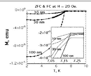
FIG. 4. Field cooled (FC) and zero field cooled (ZFC) magnetization vs temperature of lead grains of sizes 100, 30, and 10 nm. The critical temperature is unchanged within the experimental accuracy. Note that the magnetization is not normalized per weight. Inset: blowup of the transition region.
