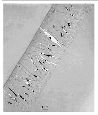
FIG. 2. TEM micrograph for 50 nm NP membrane, slice perpendicular to the membrane.
