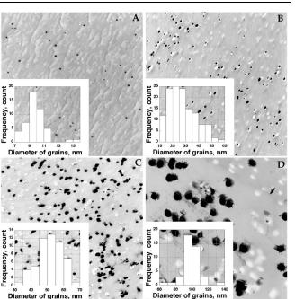
FIG. 1. TEM micrographs, slices parallel to the membrane for (a) 10 nm NP membrane loaded with lead, (b) 30 nm NP membrane, (c) 50 nm NP membrane, and (d) 100 nm NP membrane. The size distribution of the particles is also presented.
