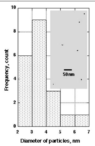
FIG. 6. Size distribution for lead particles in a 10 nm pore membrane with a loading of  $1.2 \ \mu g/cm^2$ . Inset: a contrast enhanced TEM micrograph of these particles in a  $\approx 50$  nm slice parallel to the membrane surface.
