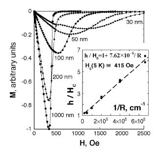
FIG. 3. Normalized magnetization vs *H* at 5 K according to Eq. (1) for different pore size NP membranes loaded with lead. Inset: normalized critical fields  $h/H_c$  vs 1/R (see text).
